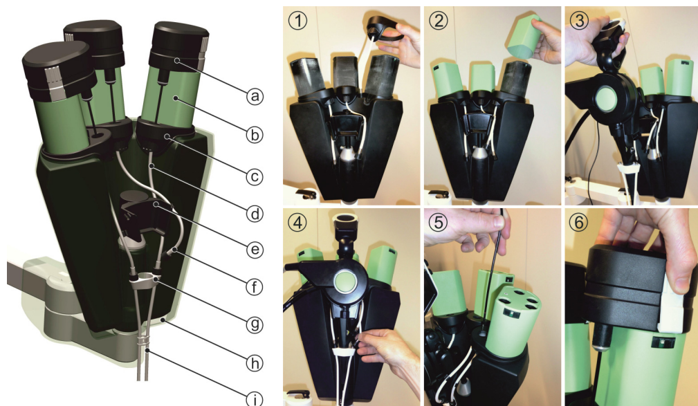
Figure 5.12 Sterile parts and installation instruction of the robotic shaft manipulation module: (a) Instrument, (b) Sterile sleeve column, (c) Sterile adapter working channel drive unit, (d) Working channels drive unit steerable instrument, (e) Docking station, (f) Working channel drive unit non-steerable instrument, (g) Sterile adapter working channel endoscopic platform, (h) Sterile sleeve, (i) Working channel endoscopic platform, (1-6) Installation instruction
