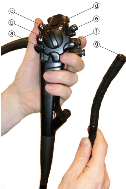
Figure 3.6 Control section endoscope: (a) Navigation wheel left-right, (b) Lock navigation wheel left-right, (c) Navigation wheel up-down, (d) Programmable switches, (e) Lock navigation wheel up-down, (f) Valves for insufflation, rinsing, and suction, (g) Steerable tip with camera
