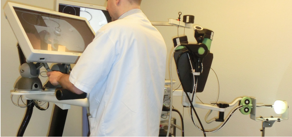
Figure 6.1 Experimental setup for clinical experts to test the full robotic flexible endoscope
