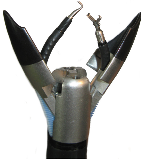
Figure 1.8 The ANUBIS NOTEScope® (©Karl Storz). The tip opens in the operating field to expose two instruments both with 4 degrees of freedom and controlled with pistol like handles [Bardou et al., 2009]
