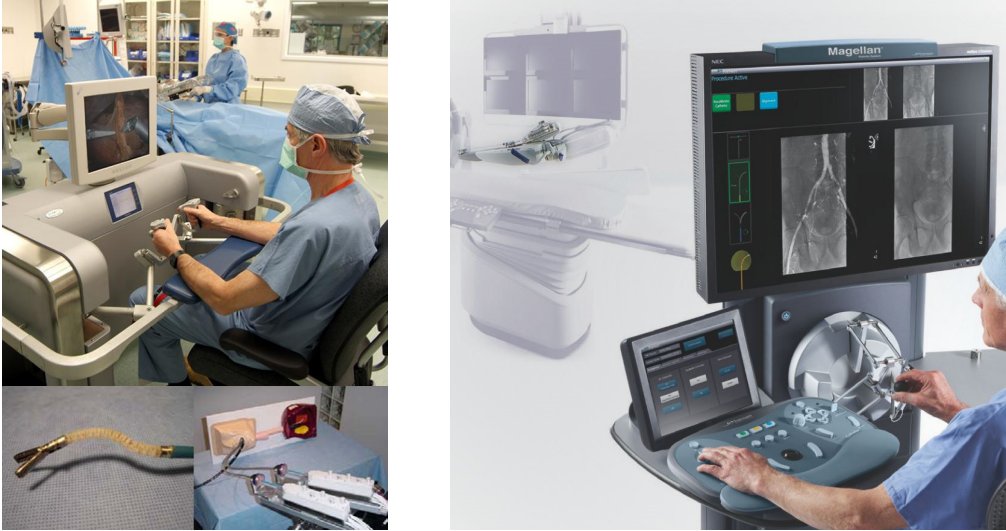
Figure 1.12 (a) ViaCath® robot (left) [Abbott et al., 2007]; (b) Magellan® robotic catheter (right, © Hansen Medical)
