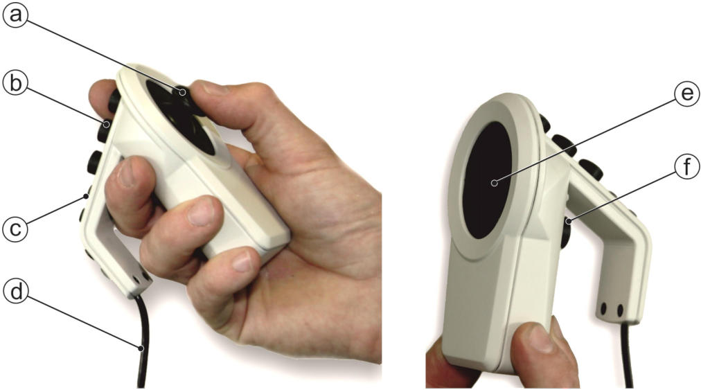
Figure 3.14 Joystick and touchpad remote controllers: (a) Thumb joystick, (b) Buttons for insufflation, rinsing, and suction, (c) Programmable switches, (d) USB cable to computer, (e) Touchpad, (f) Hold-to-run safety switch.
