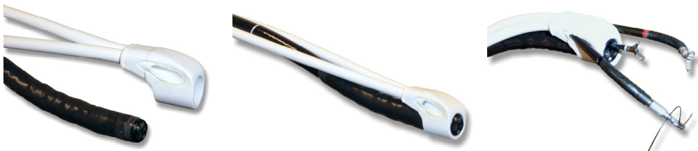
Figure 5.13 Cap for instrument guidance endoscopic platform: (left) Cap with instrument channels attached, (middle) Cap positioned on gastroscope, (right) Two steerable instruments and one non-steerable instrument protrude from the tip.
