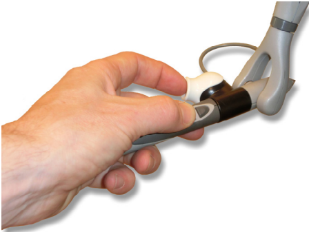
Figure 5.17 Stylus pen of the multi-DOF controller, including the standard buttons and the index finger joystick that is developed within this project
