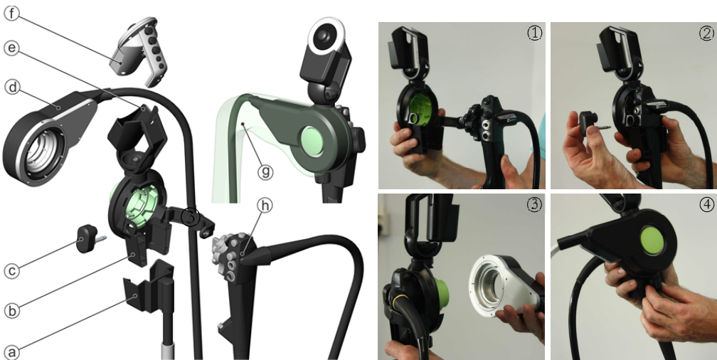
Figure 3.12 Exploded view and installation instruction of the robotic steering module: (a) Docking station, (b) Interface unit, (c) Plug, (d) Drive unit, (e) Holder remote control, (f) Remote control, (g) Sterile sleeve, (h) Endoscope, (1-4) Installation instruction
